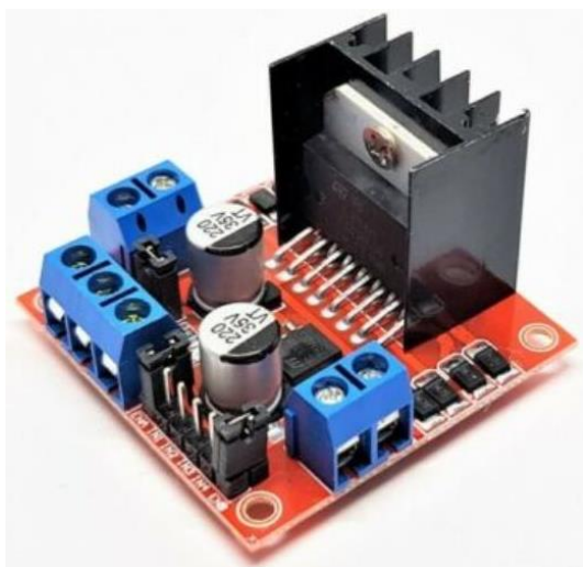
Figure - Dual H Bridge DC Stepper Motor Drive Controller Board Module L298N
