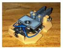
3.5mm audiojack receptacle goes on keyer-base from rear side. Use receptacle which has body length around 13mm.
